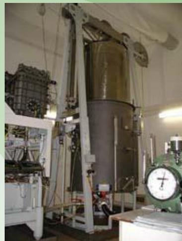
In comparison with verification against standard gas meters this method is not so productive but is more accurate and reliable due to the strictly defined constant volume in contrast to standard gas meters that have some uncertainty of measurement and reproducibility. For the reason stated it can be also used as standard equipment for the verification of standard gas meters.
